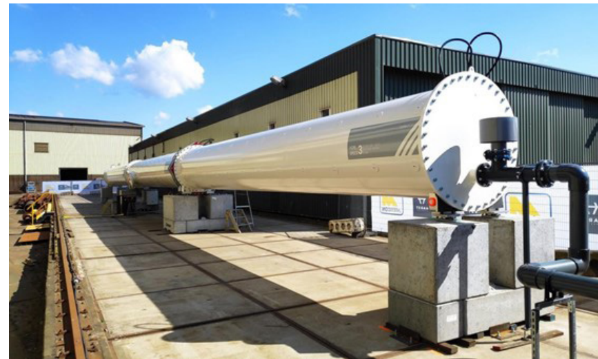
Figure 27: Photo of the INPR in operational state and attached to the vacuum pumps.
