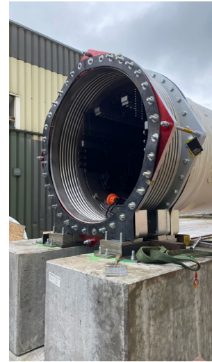
Figure 25: Photo of the expansion joint.
