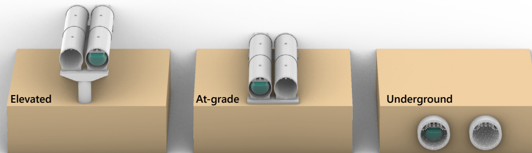
Figure 11: A conceptual visualization of hyperloop infrastructure implementation topologies: elevated, at-grade and underground.
